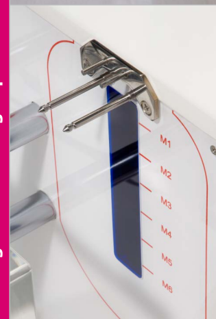
12 M-Sensors keep buffy coat on the right level during separation
